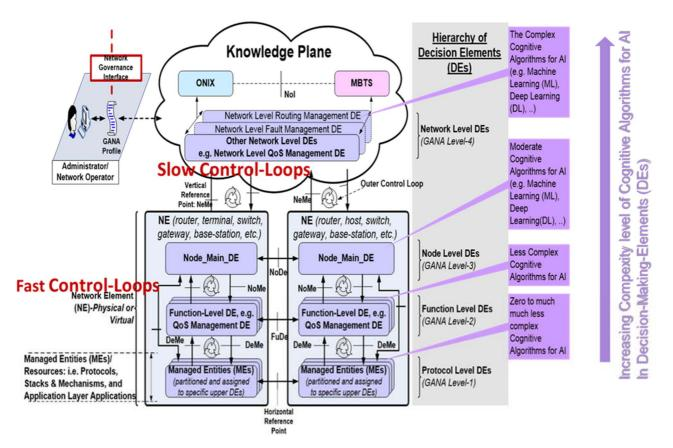
Figure 1: Snapshot of the GANA Reference Model and Autonomics Cognitive Algorithms for Artificial Intelligence (AI)
