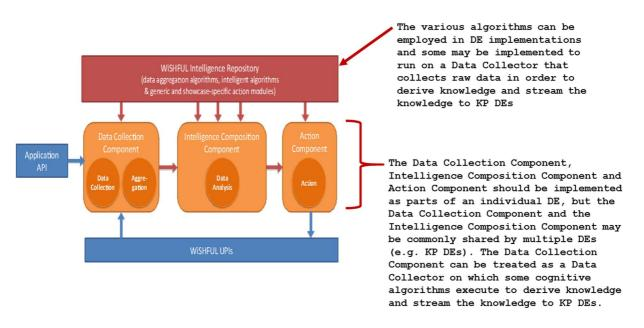
NOTE: This figure also provides insights on the various algorithms that can be employed in DE implementations while some algorithms may be implemented on Data Collectors.
