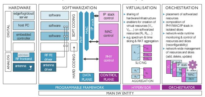
Figure 9: Illustration of Softwarization, virtualization and orchestration principles in the H2020 ORCA project
